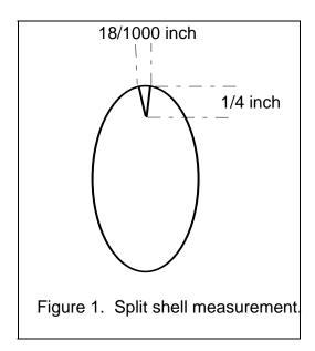
When it is questionable as to whether or not a shell should be scored as non-split, the opening should be checked with a feeler gauge of the proper dimensions. The gauge should not be forced into the opening. Shells having splits smaller than the required opening shall be scored against the restricted tolerance for "non-split" as shown in line (a) (1) of Table I in the grade standards.
